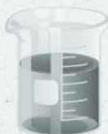
Beaker 5 750 mL Distilled H 2 O 10mg fertilizer
